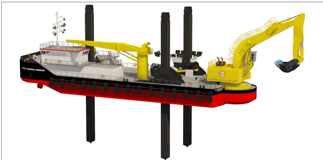
Figure 2: Typical Backhoe Dredge
