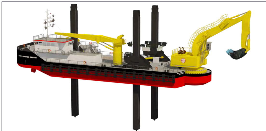
Figure 2: Typical Backhoe Dredge
