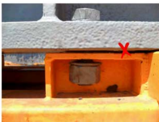
All mounting bolts must be tightened prior to despatch.
