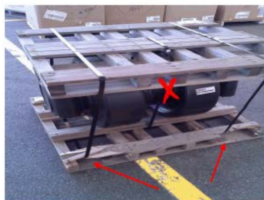
No weight on the boards has caused them to pull during transit and handling.
